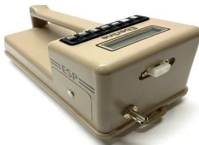
Figure 2. Portable scintillation detector system used for outdoor gamma dose rate measurements
