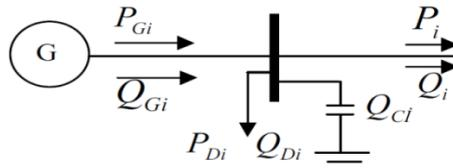
Figure 1. Sketch of a general purpose bus
