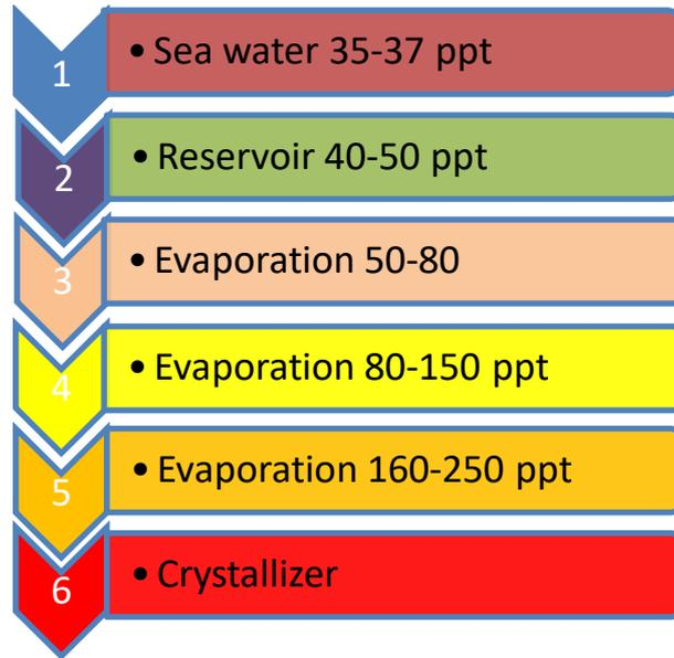
Figure 4. The common salt production system on salt fields
