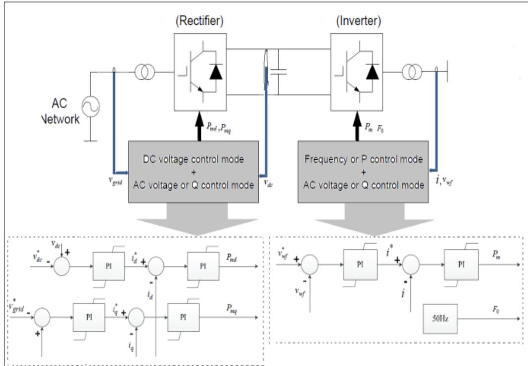
Figure 2. Overall control structure of the VSC-HVDC
