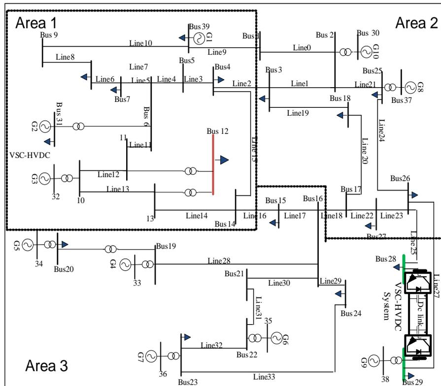
Figure 7. IEEE 39 bus test system with VSC-HVDC
