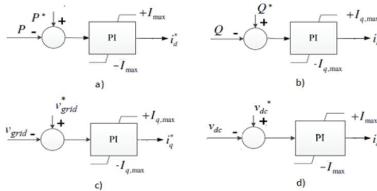
Figure 5. Outer controllers a) Controllers PI controller for active power control b) Controllers PI controller for reactive power control c) Basic scheme for AC control d) Controllers PI controller for active power control
