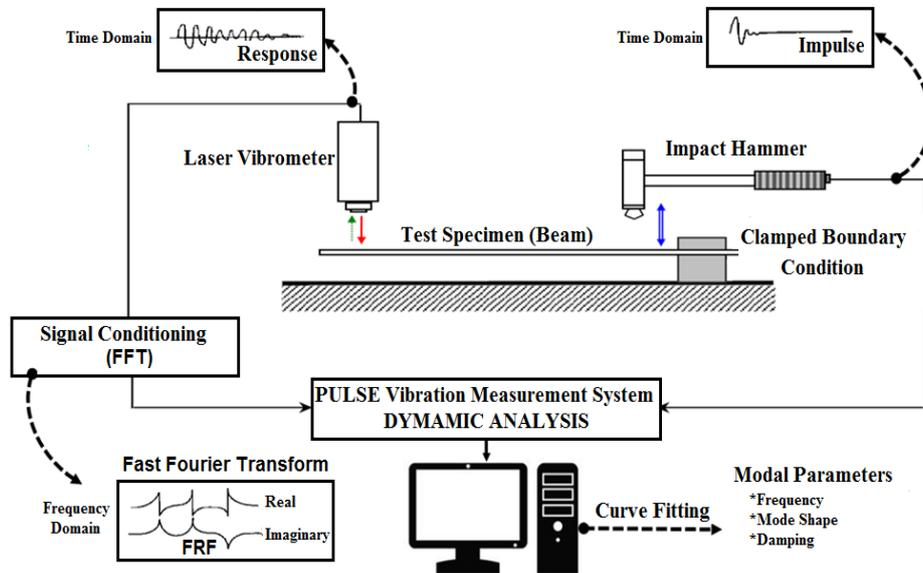
Figure 1. Schematic representation of vibration testing system
