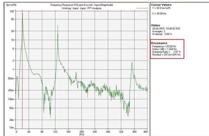
Graphic 4. Schematic presentation of first natural frequency and damping ratio
