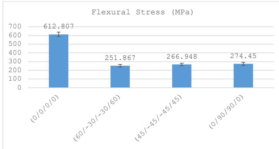
Graphic 2. Maximum flexural stress of composite samples
