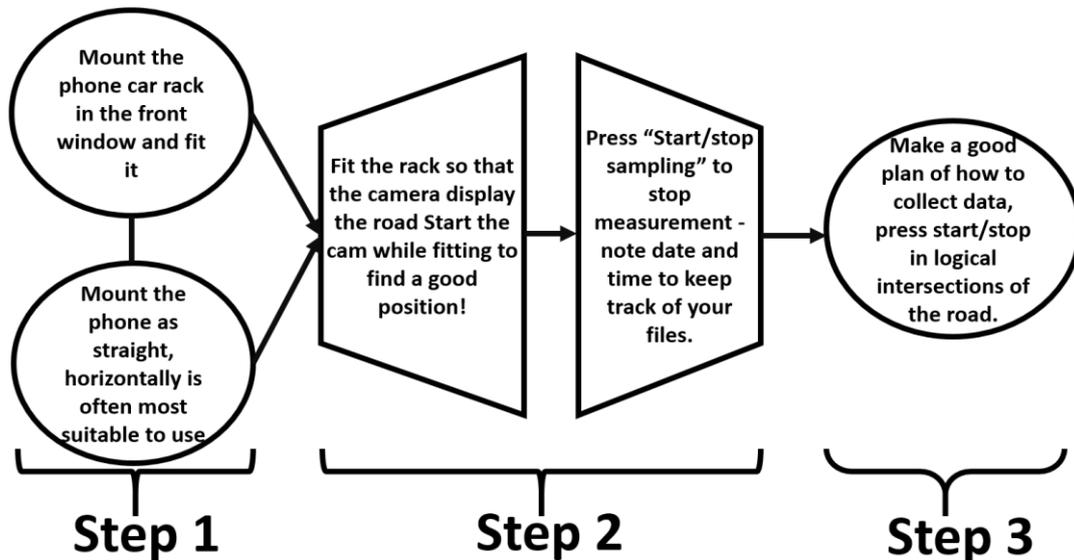
Figure 4. Installation of roadroid system into the car
