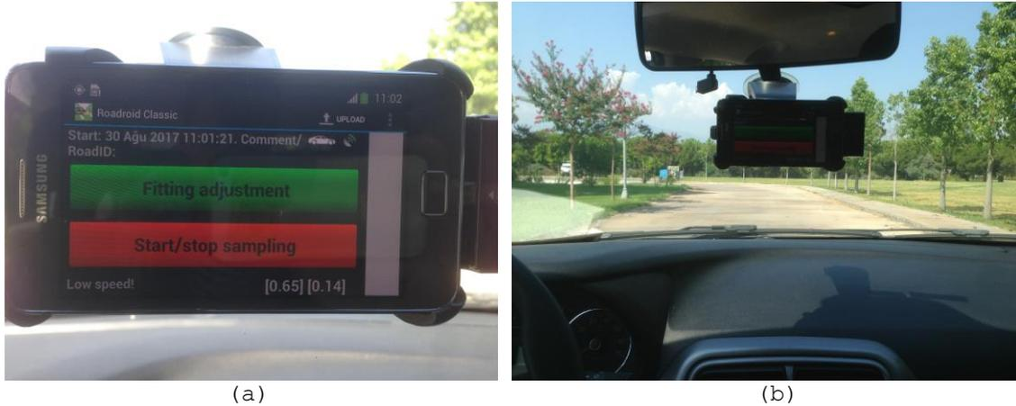
Figure 3. Used Galaxy S2 smartphone with roadroid road roughness measurement application
