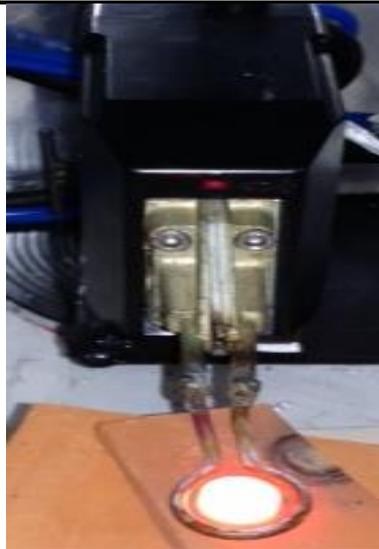
Figure 2. Induction sintering process of the iron based PM compact
