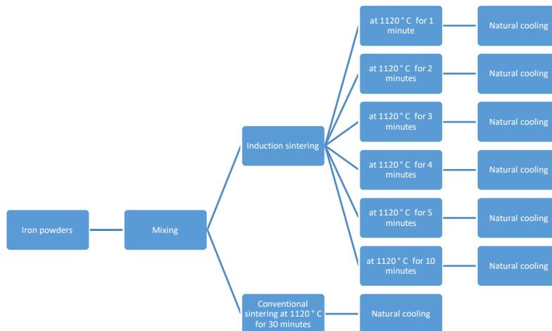
Figure 4. Flow chart of the sintering process
