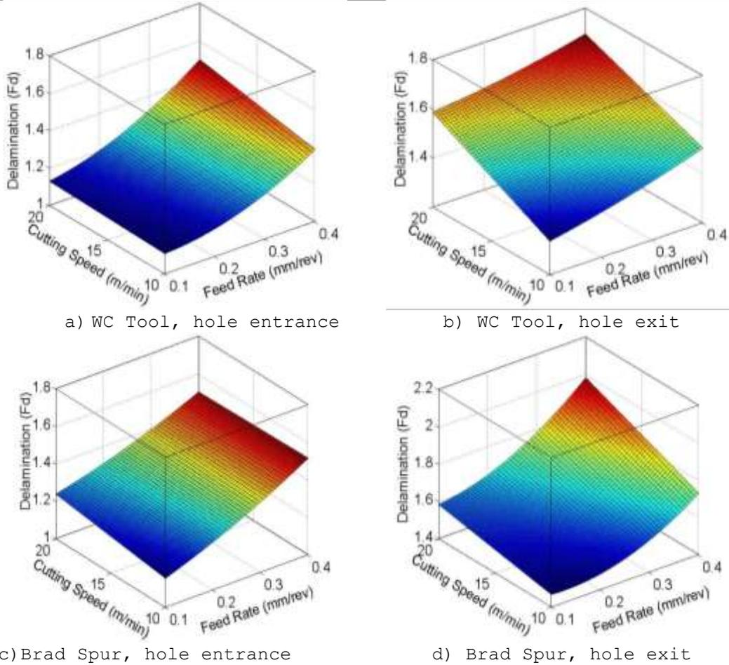
Figure 4. The effect of feed rates and cutting speeds on delamination
