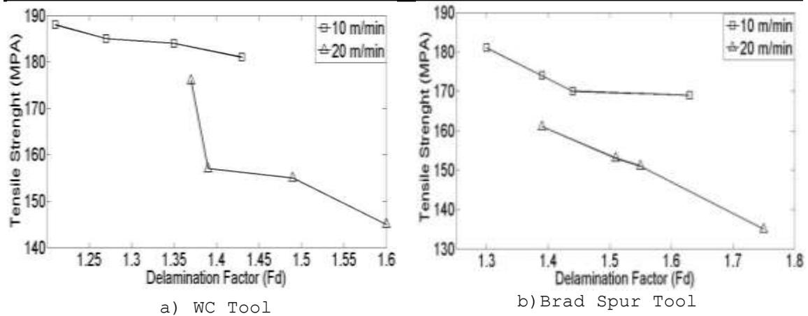
Figure 5. The effect of delamination on tensile strength
