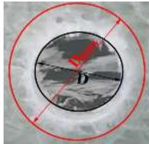
Figure 2. Delamination area on the hole
