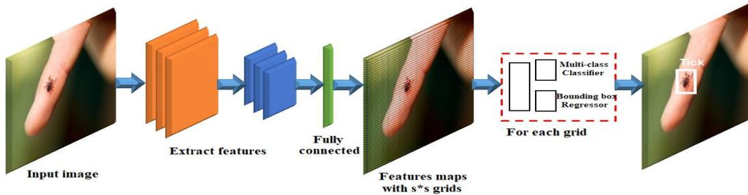
Figure 2. Yolo-v3 model diagram used in tick detection
