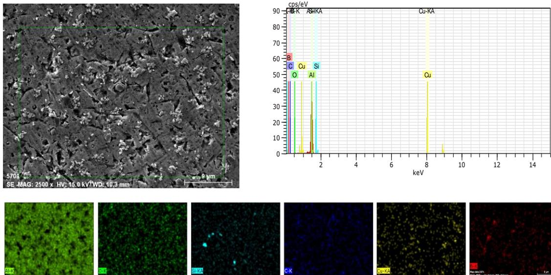
Figure 1. EDX analysis of Al2024 matrix composites reinforced with wt. 2% SiC-B<sub>4</sub>C hybrid nanocomposite bulk sample
