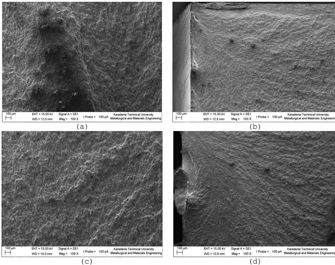
Figure 3. SEM image of bending strength fracture surface (a)Al2024, (b)Al2024/wt.2% SiC-B<sub>4</sub>C hybrid nanocomposite and SEM image of tensile strength fracture surface (c)Al2024, (d)Al2024/wt.2% SiC-B<sub>4</sub>C hybrid nanocomposite samples
