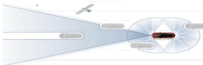
Figure 16. Lane change and radar coverage, camera, and ultrasonic sensor.
