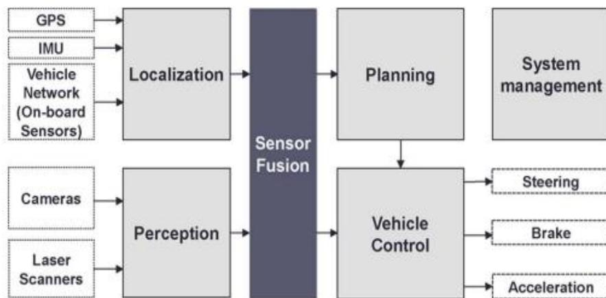
Figure 1. Fundamental functions of autonomous vehicle [1]
