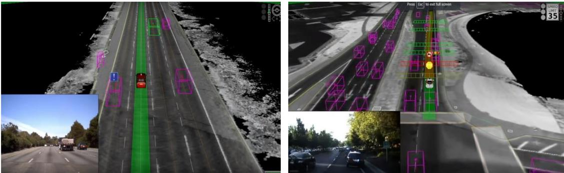
Figure 14. a) Identification of heavy vehicles; b) Recognition of the police cars [14]
