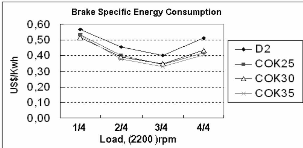
Figure 5. The variation of the brake specific energy consumption for different blended fuels with 2200 rpm fixed engine speed and various throttles opening position.
