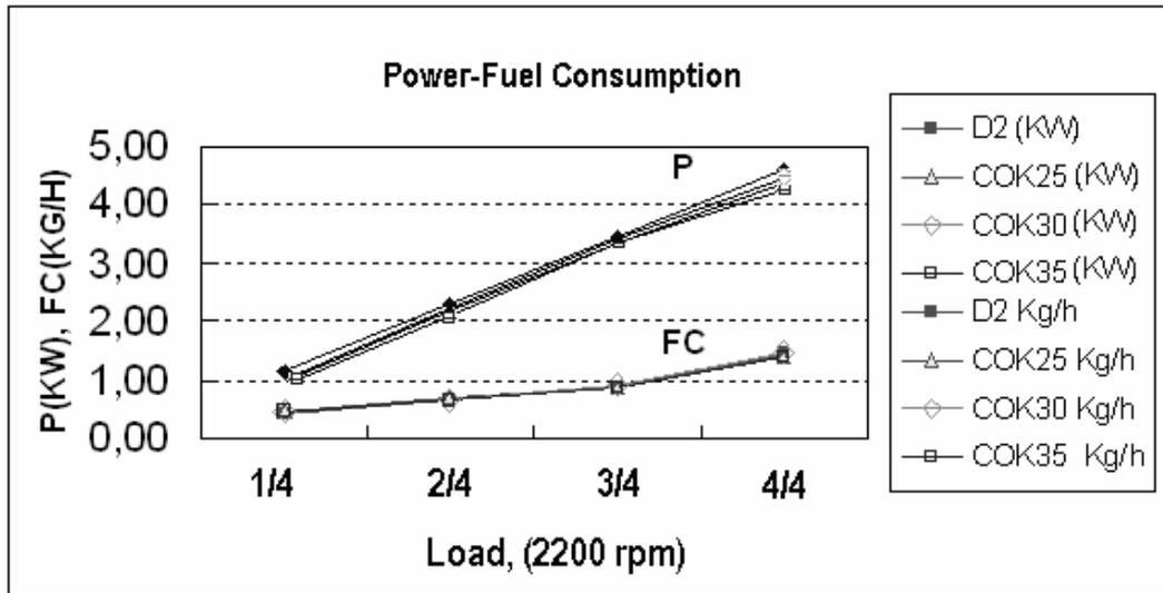
Figure 2. The engine power of test engine using different blended fuels under various throttle opening positions
