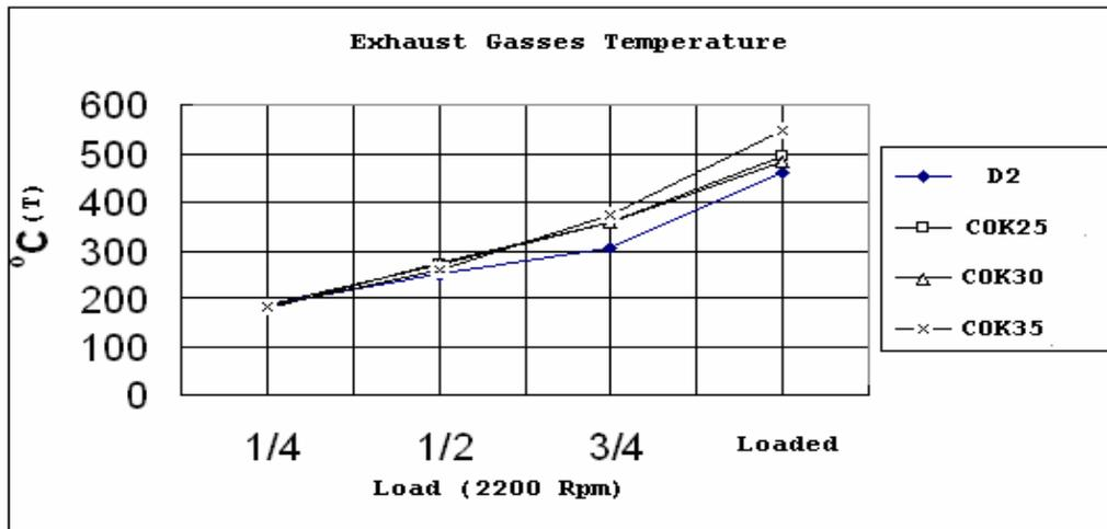
Figure 4.Variation of the Exhaust gasses temperature of the engine using different blended fuel in comparison to D2.
