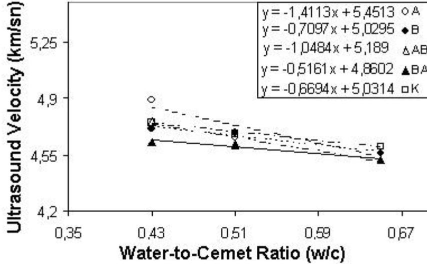
Figure 4. The variation of ultrasound velocity with w/c ratio
