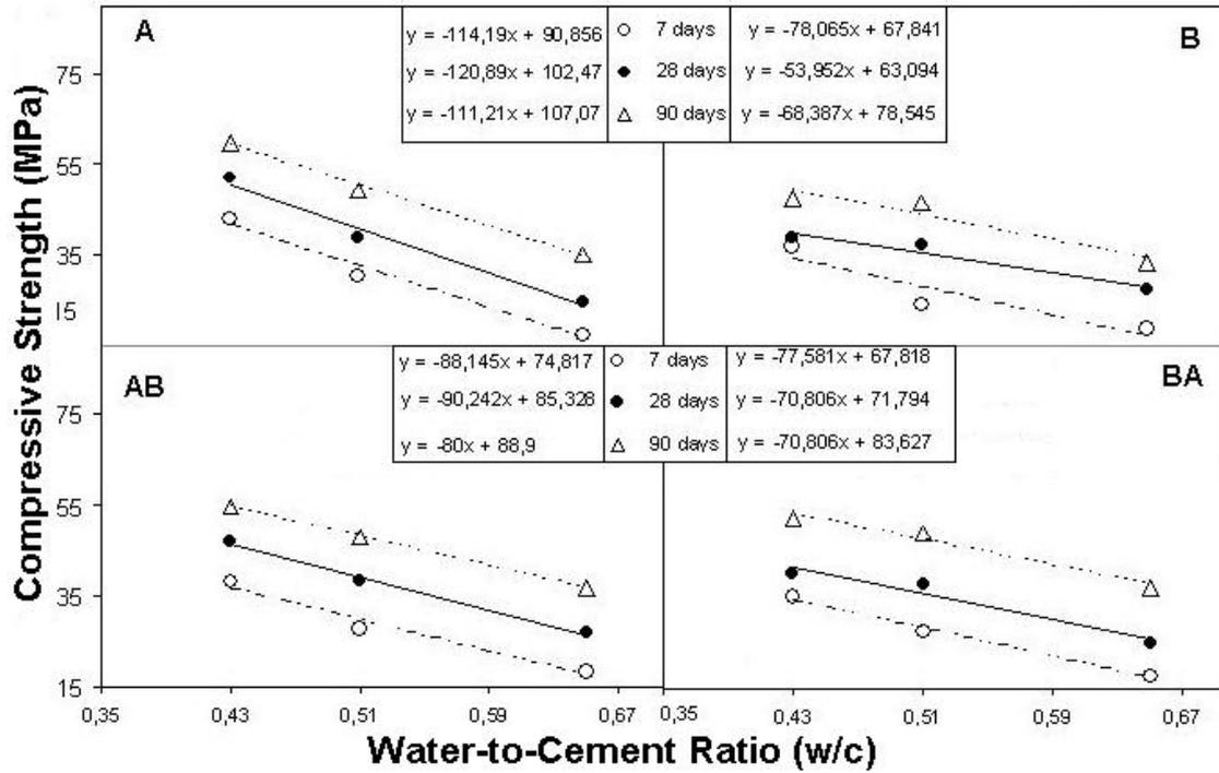
Figure 1. The variation of Compressive Strength with the w/c ratio in different types of concretes
