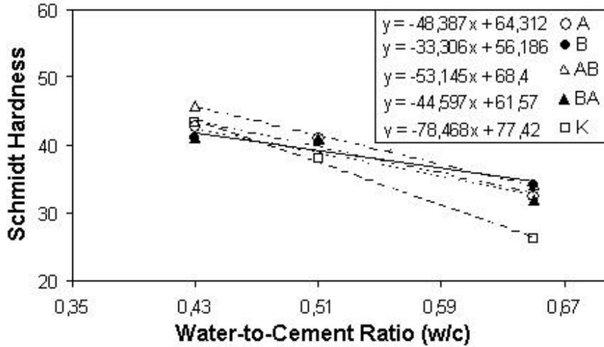
Figure 2. The variation of Schmidt hardness with w/c ratio
