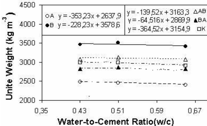
Figure 3. The variation of unit weight with w/c ratio
