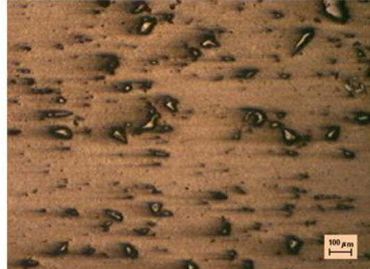
Figure 3. 15 % FeB<sub>x</sub> particles in the Al Matrix.
