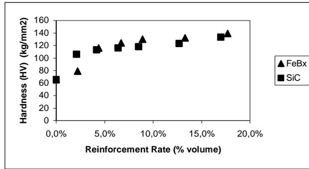
Figure 11. The effect to hardness of reinforcement rate (volume %)
