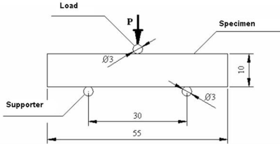
Figure 1. Mechanism of three points bend test
