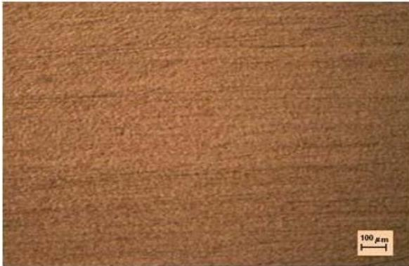
Figure 2. 100% Al powder metal specimen.
