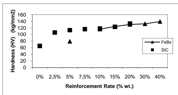
Figure 10. The effect to hardness of reinforcement rate (wt. %)
