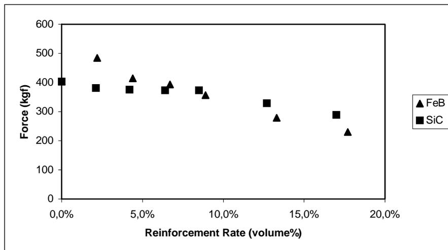
Figure 13. The effect to three point bend strength of reinforcement rate (volume %)
