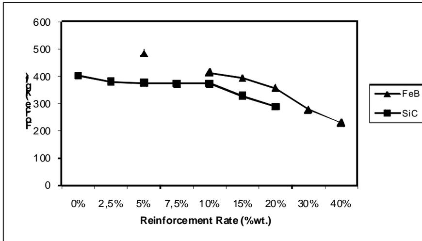
Figure 12. The effect to three point bend strength of reinforcement rate (wt%)
