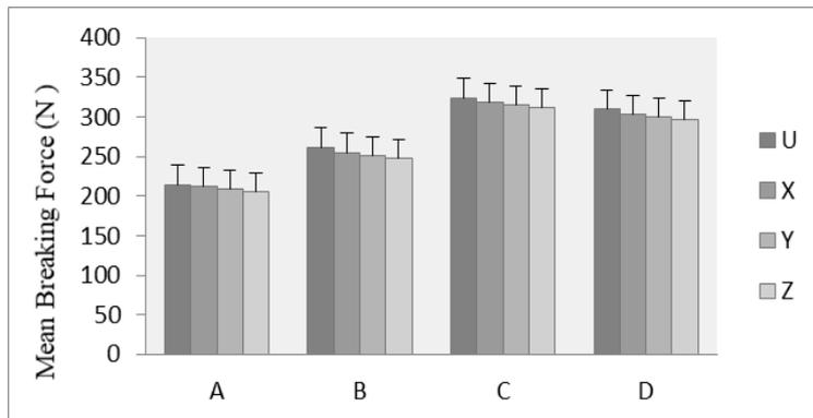
Figure 5. Tensile strength (strip method) in weft direction for untreated and treated fabric samples
