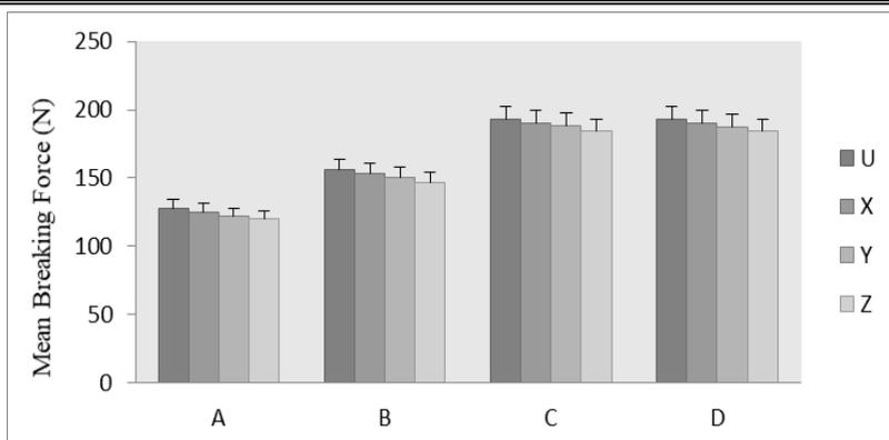
Figure 7. Tensile strength (grab method) in weft direction for untreated and treated fabric samples
