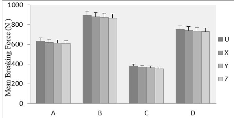
Figure 4. Tensile strength (strip method) in warp direction for untreated and treated fabric samples
