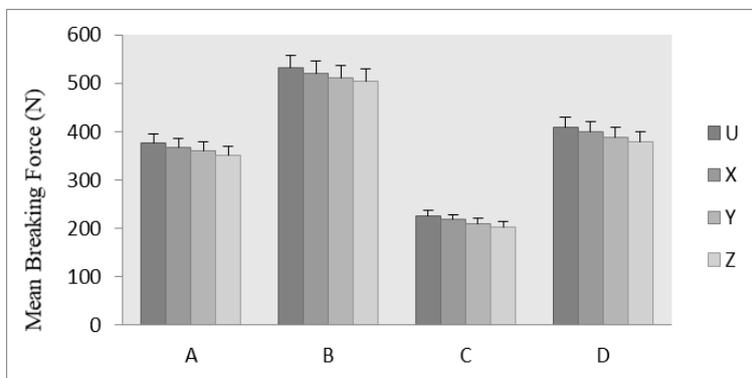
Figure 6. Tensile strength (grab method) in warp direction for untreated and treated fabric samples
