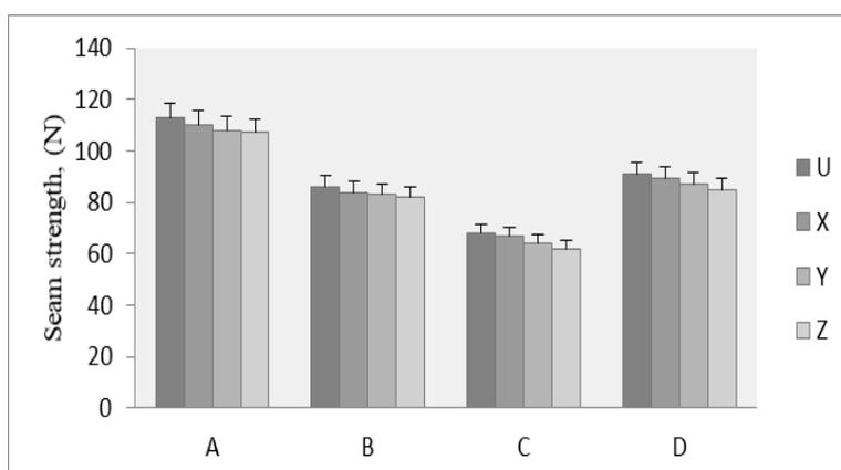
Figure 10. Seam strength in warp direction for untreated and treated fabric samples
