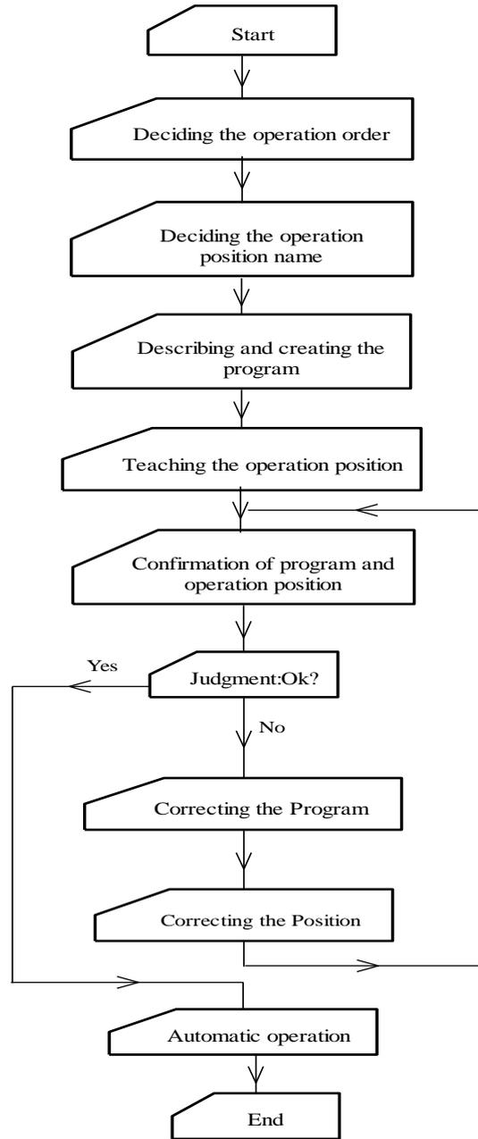
Figure 4. Flow chart of robot application process
