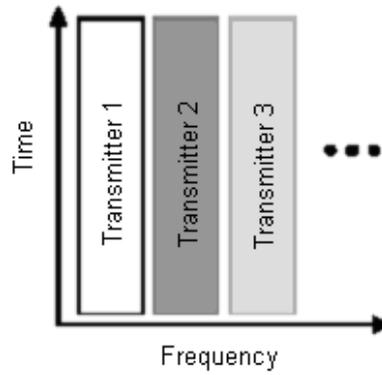
Figure 4 Time-frequency characteristic of FDMA
