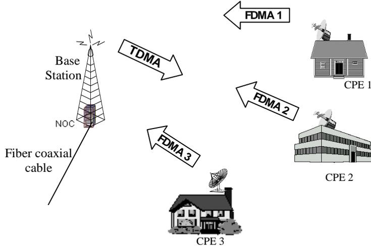
Figure 2. Typical LMDS architecture
