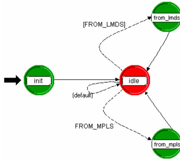
Figure 7. BASE station MPLS module process model.
