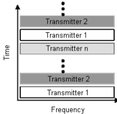
Figure 3. Time-frequency characteristic of TDMA
