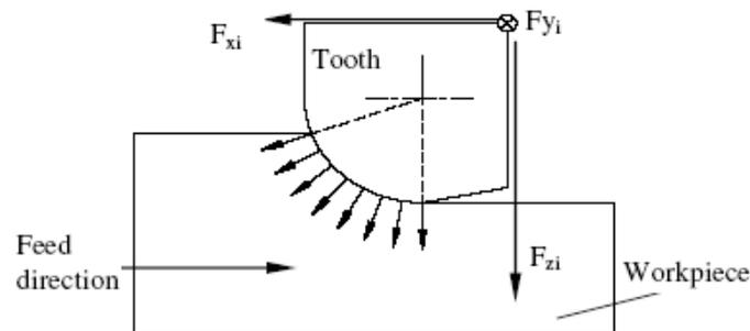
Figure 2. Distribution of vectors of cutting forces on x-z plane
