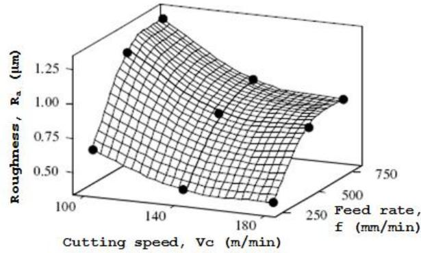
Figure 5. Effect of cutting parameters on surface roughness
