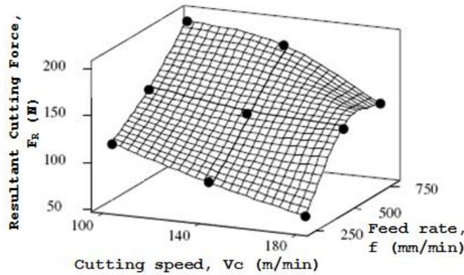
Figure 3. Effect of cutting parameters on resultant cutting force
