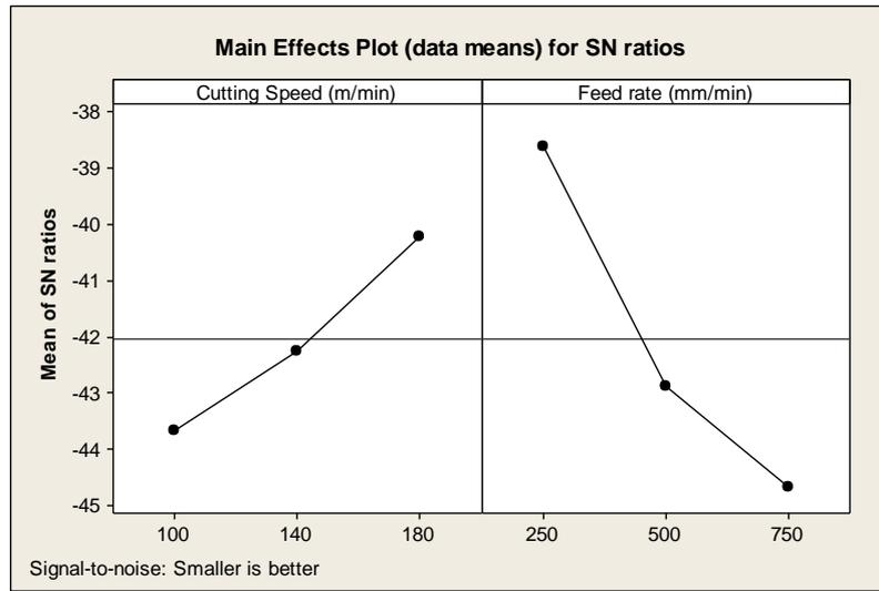
Figure 4. Main effect plot for S/N ratio of  $F_R$
