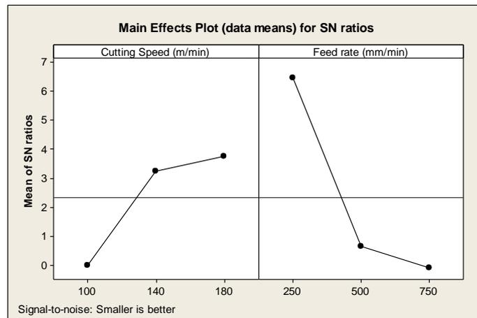
Figure 6. Main effect plot for S/N ratio of  $R_a$
