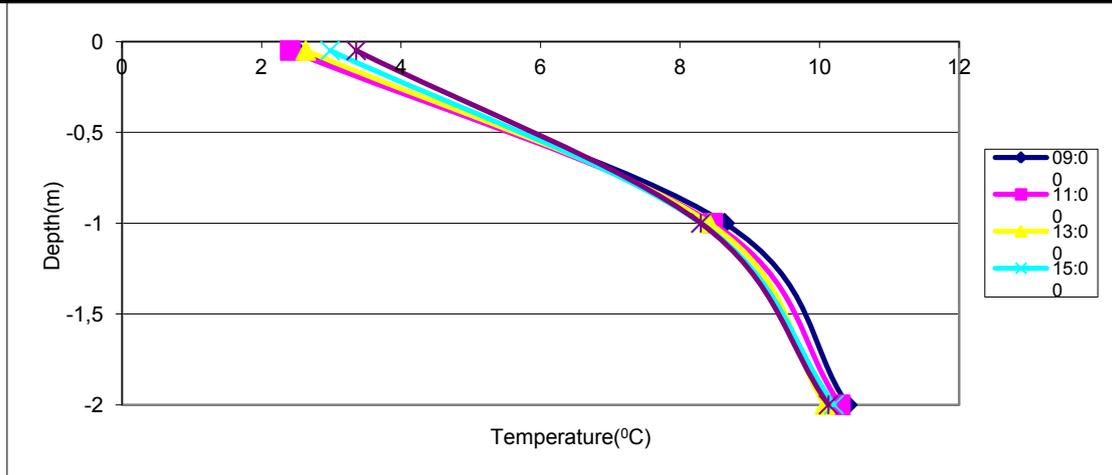
Figure 8. Temperature changes in soil of horizontal slinky ground heat exchanger hole
