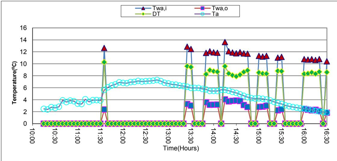
Figure 7. Temperature changes of  $T_{wa,i}$ ,  $T_{wa,o}$  and  $T_a$  in time
