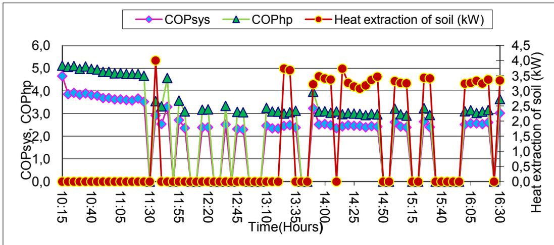
Figure 5. The change of  $COP_{sys}$ ,  $COP_{hp}$  and the heat extraction of soil in time
