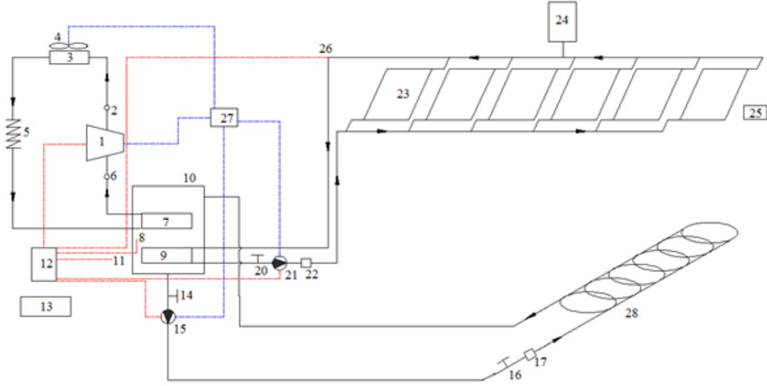
Figure 3. The detailed schematic diagram of Solar and Ground source heat pump system
