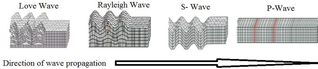
Figure 3. Types of seismic waves
