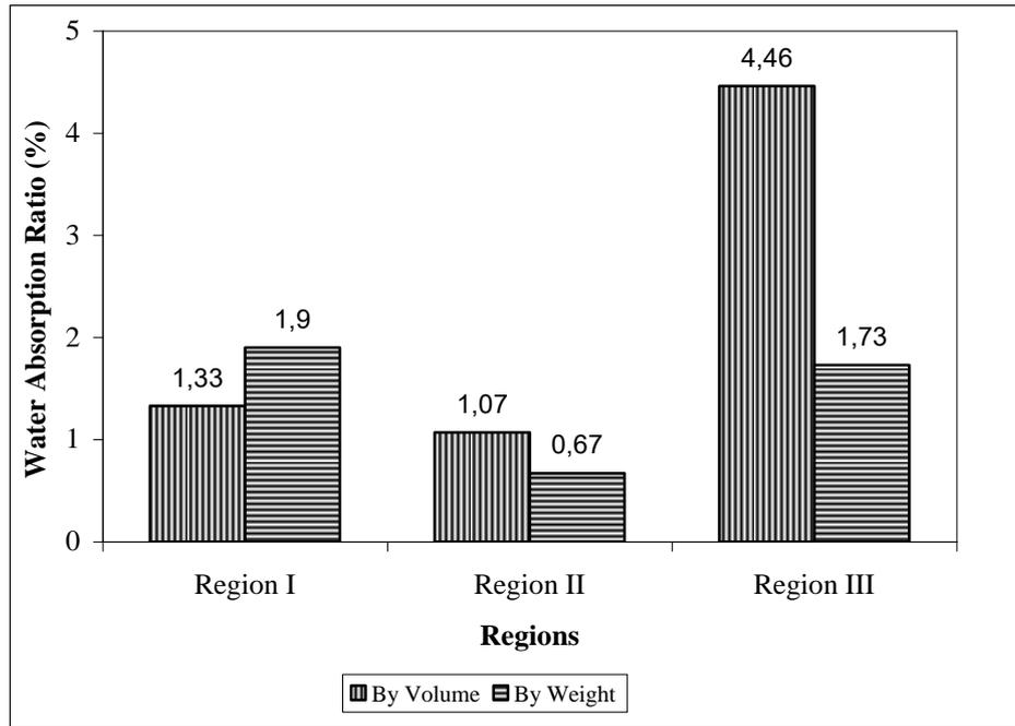
Figure 3. Water absorption ratios of the Basalt stones
