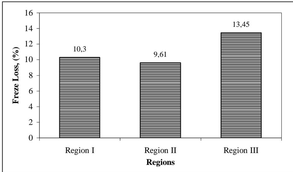
Figure 6. Freeze loss with sodium sulphate variations of the specimens
