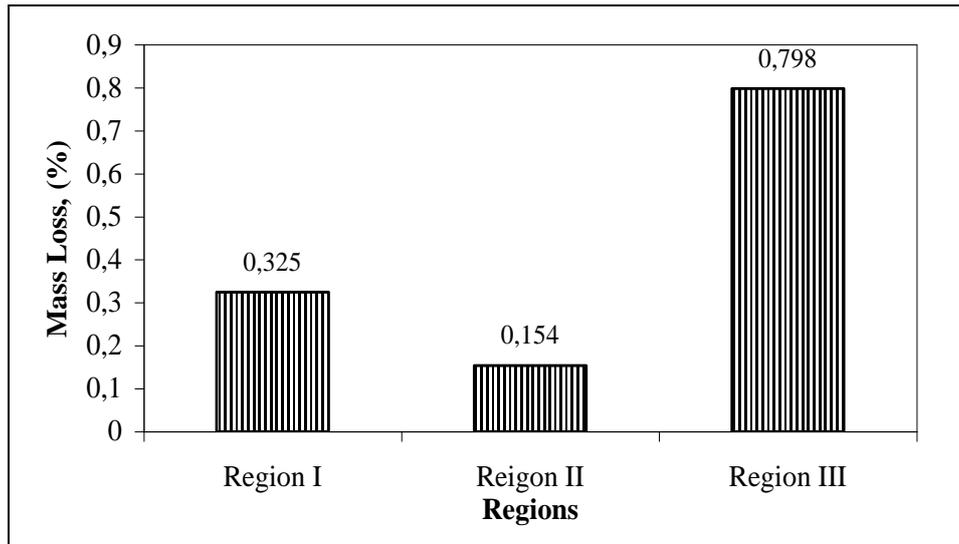
Figure 4. Mass loss variations of the specimens after freeze-thaw test
