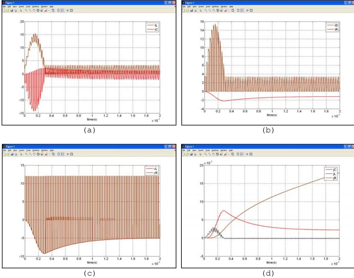
Figure 6.a) The graphs of inductance and capacitance currents, b) The graphs of diode and load currents, c) The graphs of inductance and load voltages, d) The graphs of energy alterations in R,L,C
