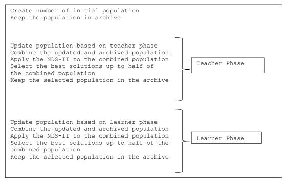
Figure 5. Using NDS-II with the TLBO algorithm
