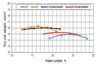
Figure 3. The effects of domestic wastewater on compaction of natural soils
