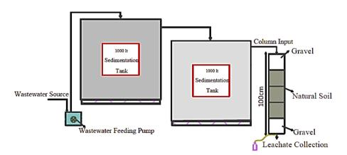
Figure 2. Schematic representation of the pilot facility (unscaled)
