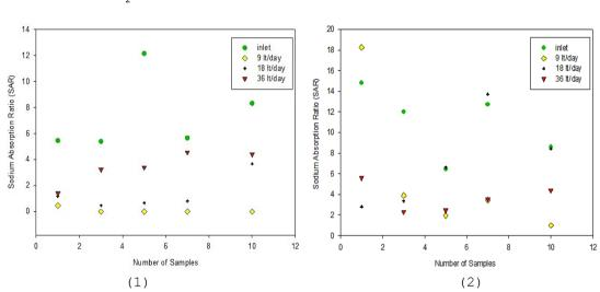
Figure 7. (1) SAR filtration of soil G (2) SAR filtration of soil K
