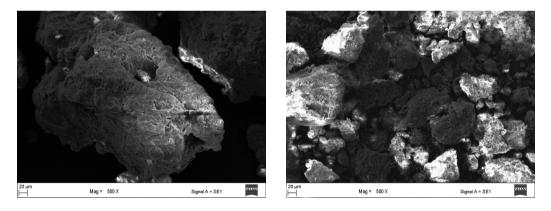
(1) (2) Figure 5. Sem image of G natural soil (1) uncontaminated soil (2) contaminated soil
