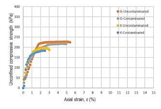
Figure 4. The effects of domestic wastewater on UCS of natural soils
