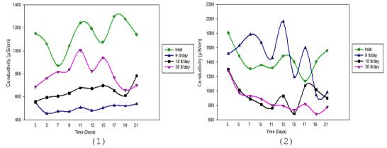
Figure 11.(1) Conductivity filtration of G soil-column(2) Conductivity filtration of K soil-column
