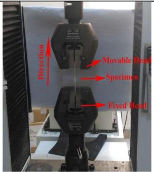
Figure 3. Tensile test setup
