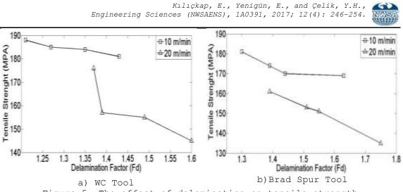
Figure 5. The effect of delamination on tensile strength
