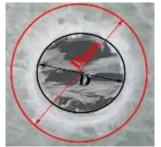
Figure 2. Delamination area on the hole
