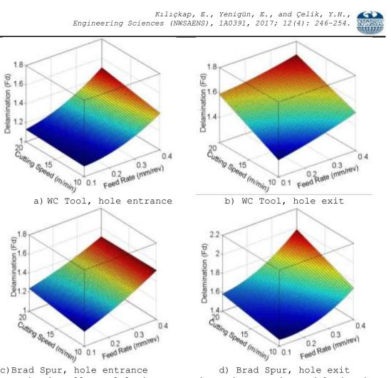
c)Brad Spur, hole entrance d) Brad Spur, hole exit Figure 4. The effect of feed rates and cutting speeds on delamination
