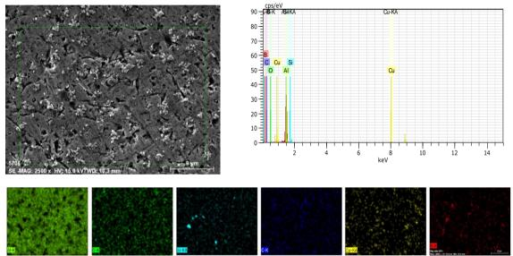
Figure 1. EDX analysis of Al2024 matrix composites reinforced with wt. 2% SiC-B4C hybrid nanocomposite bulk sample
