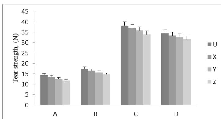
Figure 8. Tear strength in warp direction for untreated and treated fabric samples
