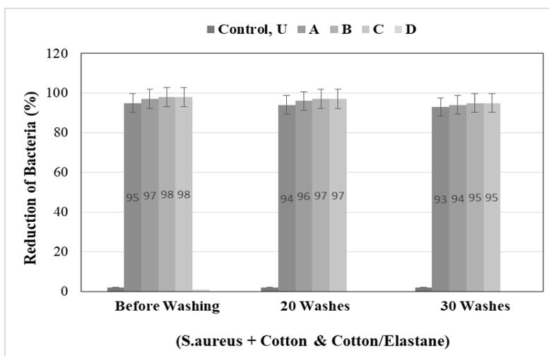
Figure 3. Antimicrobial test results of the control and triclosan bound with cotton samples
