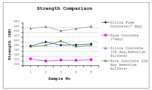
Figure 1. Comparison of 7-28 day strength of silica fume and pure concrete samples
