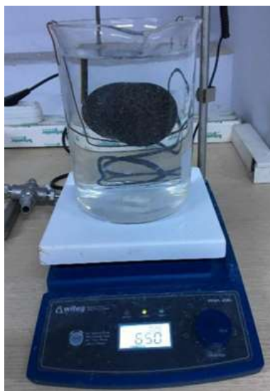
Figure 3. The dissolution of NaCl particles with magnetic stirrer hot plate
