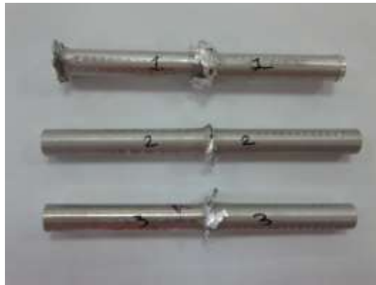
Figure 2. Overview of friction welded AZ63 magnesium alloys
