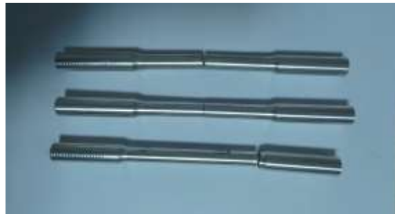
Figure 5. Optical macro-photo of tensile test results of friction-welded joints
